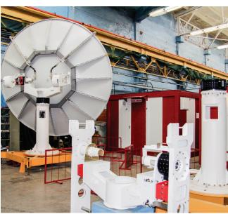
"DMRL-10" Antenna System with Gearless Synchronous Motors
