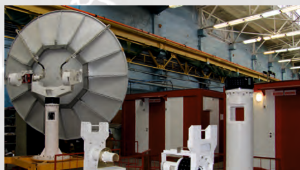
“DMRL-10” Antenna System with Gearless Synchronous Engines
